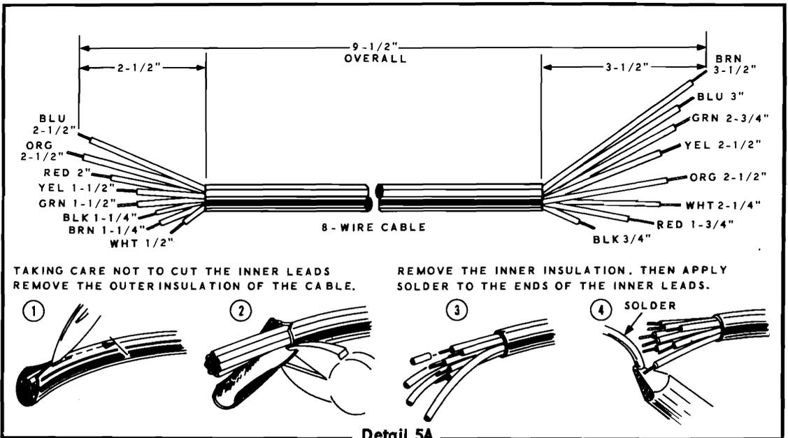
NOTE: When installing prepared cables, apply only enough heat to make a good solder connection. Excessive heat will melt the insulation on the wires.
