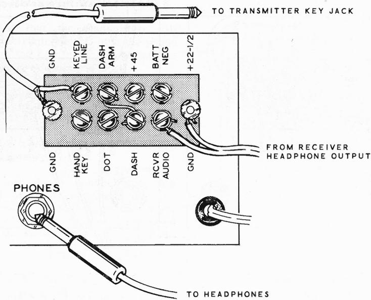
ALTERNATE USE WITH ELECTRONIC KEYSER USED AS MONITOR
