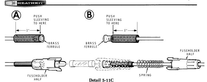
Refer to Part B of Detail 5-11C and place another 1" piece of medium (heal-shrinkable) sleeving onto the remaining 7" fuseholder wire. Slide the sleeving down until it just touches the brass ferrule.
