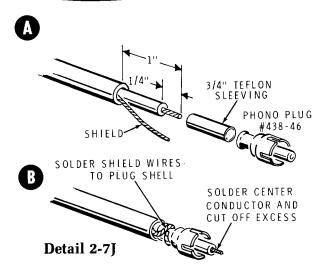
(\*\*) Refer to Detail 2-7J and install a phono plug (\*\*438-46) on end A of this cable as shown. Be sure to slide a 3/4" length of teflon sleeving onto the inner lead before you install the plug.
