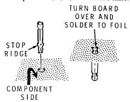
Carefully solder PCB pins B, L, and N to the foil on top of the circuit board. Keep the solder down toward the bottom part of the pins as much as possible. Connectors will be installed on these pins later.
