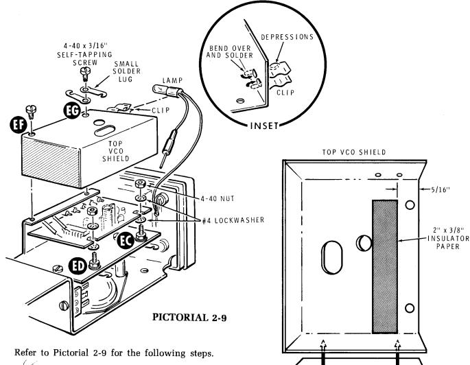
Carefully push the VCO circuit board into the shield. Then mount the board with two #4 lockwashers and a 4-40 nut at EC and ED. Be sure you do not pinch any wires between the circuit board and the shield.
