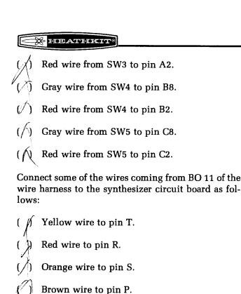
Connect the wires coming from BO 12 of the wire harness to the synthesizer circuit board as follows:
