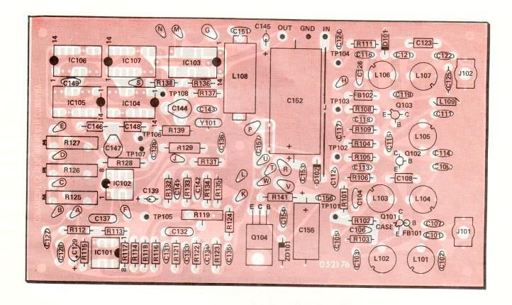
TRANSMITTER CIRCUIT BOARD (Shown from component side.
