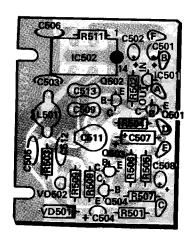
VCO CIRCUIT BOARD (Shown from component side. Foil on component side is shown in red.)
