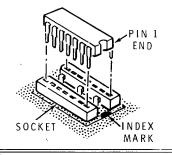
( ) IC406: MC4044P integrated circuit (#443-62).
