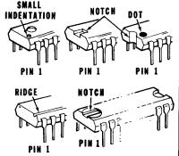
Be sure you install each IC so its pin 1 end is toward the index mark on the circuit board.
