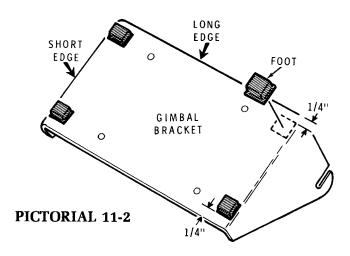
Refer to Pictorial 11-2 and turn the bracket upside down as shown. Then remove the paper backing from each of the feet and press them into place on the underside of the bracket. Be sure to keep 1/4" distance between the sides of the feet and the longer sides of ths bracket, as shown. The edges of the feet should be flush with the shorter edges of the bracket.
