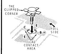
The transistor leads must be well soldered to the circuit board. A good electrical connection can be assured if you first apply a layer of solder to the lead contact areas of the circuit board foil. Once the transistors have been installed, they can be easily damaged by blows or severe jolts to the studs. Handle them with care.
