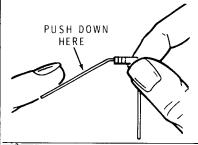
Push the leads through the holes at the indicated location on the circuit board. The end with color bands may be positioned either way.
