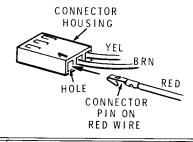
) In a like manner, insert the brown and yellow wires into the indicated holes in the connector housing.
