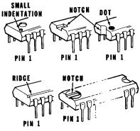
Be sure you install each IC so its pin 1 end is toward the index mark on the circuit board.
