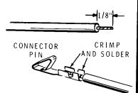
NOTE: When you perform the following step, be sure to position the connector housing and connector pins as shown before you insert the pins into the housing. Push in on the wire until the pin snaps into place.
