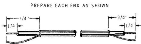
TAKING CARE NOT TO CUT THE SHIELD LEAD, REMOVE THE OUTER INSULATION.
