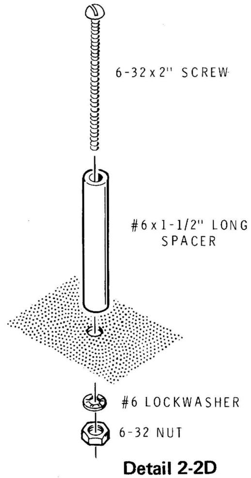
( ) Refer to Detail 2-2D and install a #6 x 1-1/2" spacer at BT. Use 6-32 x 2" hardware.
