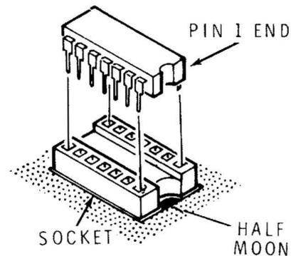
( ) IC301: SN74132N integrated circuit (#443-625).
