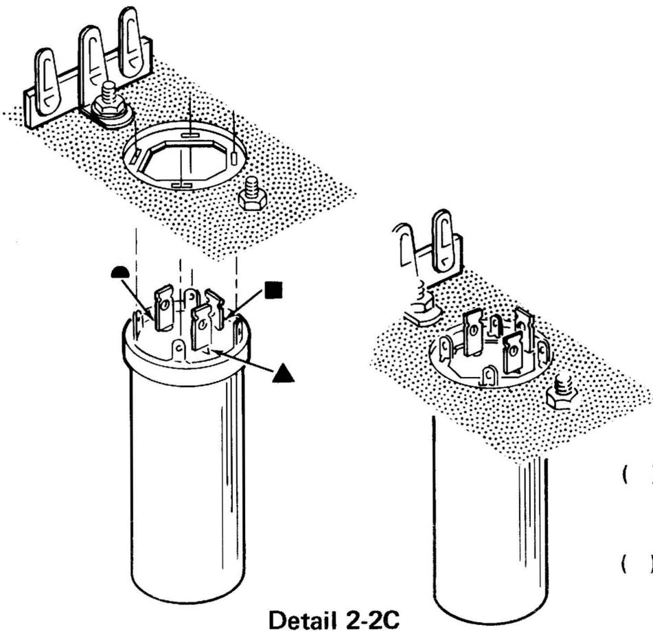
( ) C4: Refer to Detail 2-2C and mount the 100-100-300  $\mu$ F electrolytic capacitor to the capacitor mounting plate. Twist each tab 1/8 turn. Be sure to position the capacitor lugs as shown in Pictorial 2-2.
