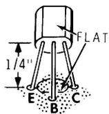
( ) Q304: MPSA20 transistor (#417-801).
