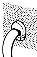
INSERT THE REAR HALF INTO THE CHASSIS HOLE.
