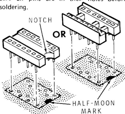
( ) 14-pin IC socket at IC301.
