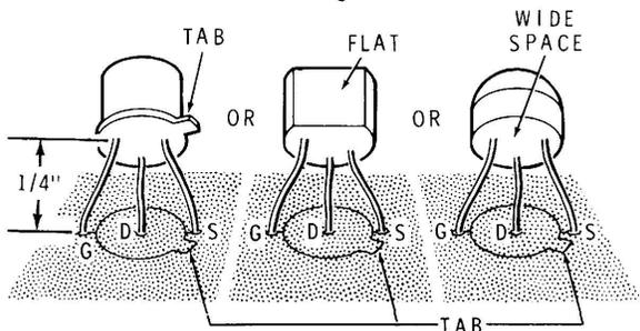
NOTE: Install the following transistors as shown. Be sure to match the E, B, and C leads on the transistor with the E, B, and C holes in the circuit board. Solder the leads to the foil as you install each transistor, and cut off the excess lead lengths.
