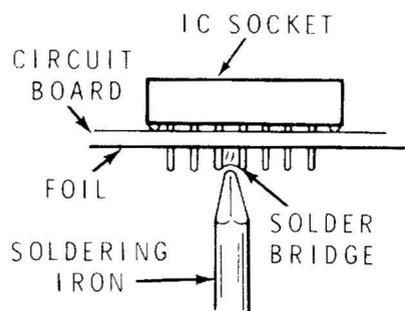
NOTE: Be sure to position the socket so the half-moon mark on the circuit board is still visible after it is installed. Solder the pins of each socket as you install it. Make sure all pins are in their holes before soldering.
