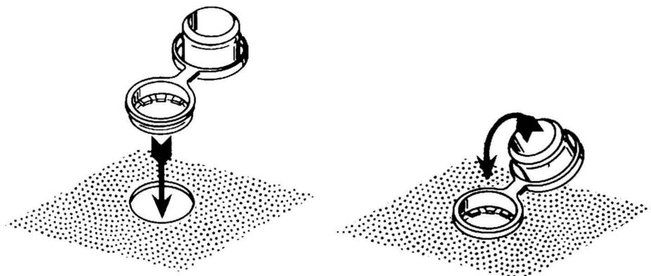
POSITION THE SMALL PORTION OF THE GROMMET INTO THE CHASSIS HOLE.
