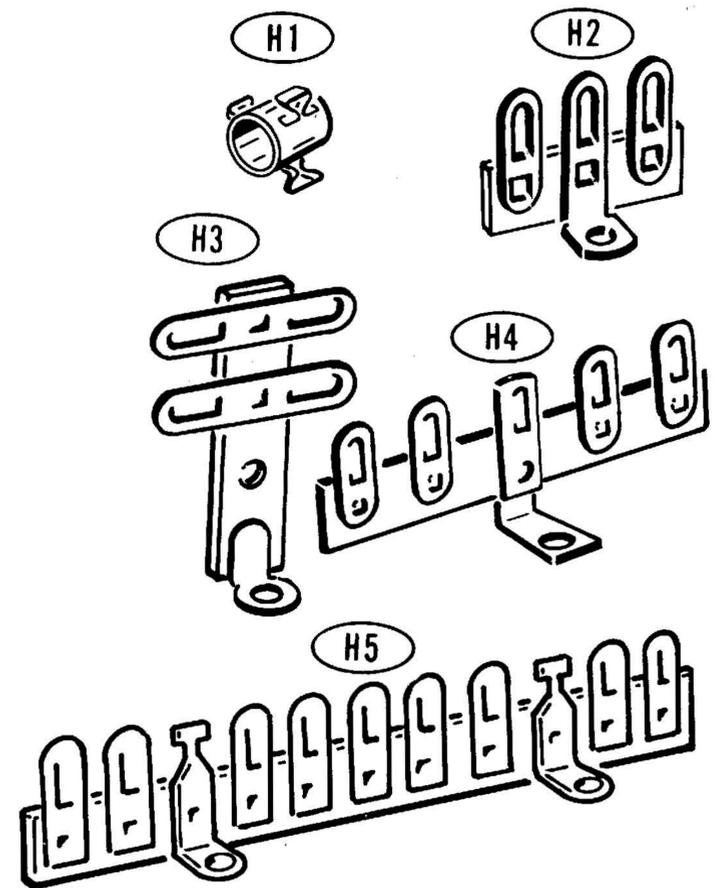
NOTE: The hardware of a particular size (stamped "#4 HDW" for example) may be in more than one packet. Open all the hardware packets of the same size hardware before you check the hardware against the Parts List.
