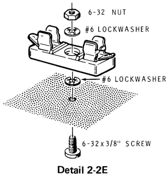
( ) Refer to Detail 2-2E and install the fuseholder at F1 with 6-32 x 3/8" hardware.
