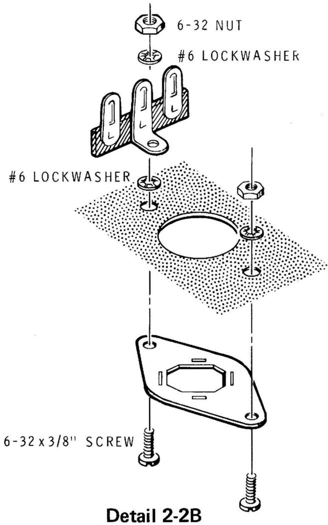
( ) Refer to Detail 2-2B and mount the capacitor mounting plate on the top of the chassis at C4 with a 3-lug terminal strip at X on the bottom of the chassis. Use 6-32 x 3/8" hardware.
